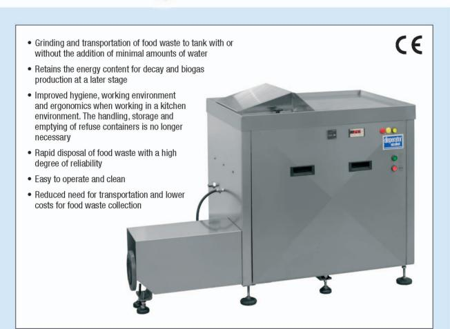
The Disperator food waste processor in the GTS-Series has been developed to meet the market's need for catering equipment for sorting at source and handling of food waste without using water as a means of transport. The system consists of two parts connected together with pipes; the food waste processor and a food waste holding tank.
